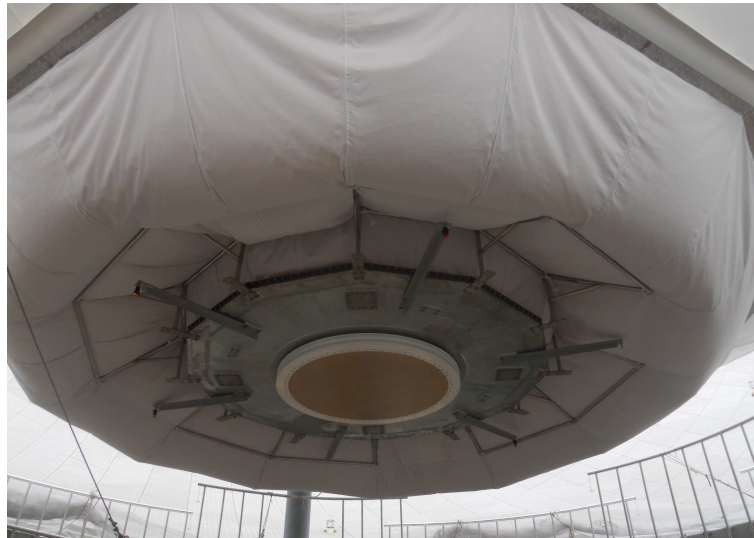
Fig. 1 The 19-beam receiver, with frequency range of 1.05 – 1.45 GHz, is installed on the lower platform of the Stewart manipulator (Stewart 1965; Yao et al. 2019), surrounded by the radiation shielding fabric.
