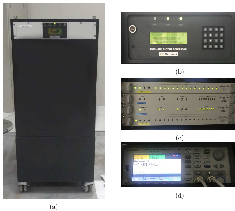
Fig. 2 The time/frequency system of FAST. (a) Hydrogen maser. (b) Auxiliary output generator. (c) Pulse distribution amplifiers for hydrogen maser and GPS. (d) Time/frequency counter.
